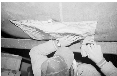
Patching a flexible belly: The technicians uses both adhesive and stitch staples to fasten a patch.
